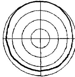
Using less of the rear signal makes a “wide cardioid,” “subcardioid” or “hypocardioid” where the rear response might be -10 or -12 dB from the front response.
