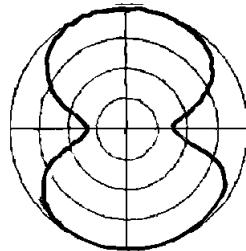
Adjusting the relative level of the front and rear allows you to control the relative sensitivity of the front and back, and also determines where the null in the pattern will be.
