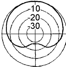
The basic pickup patterns of the two halves of the C720 are “cardioid.” Sensitivity to sound arriving from the sides, is reduced by 6 dB (half) compared with sensitivity toward the front. Toward the rear, sensitivity is reduced by 20 to 25 dB. The polar graph above shows this response. Toward the top of the page represents the direction in front of the microphone. Each half of the C720 has this directional pattern; one is facing forward and the other faces to the rear.
