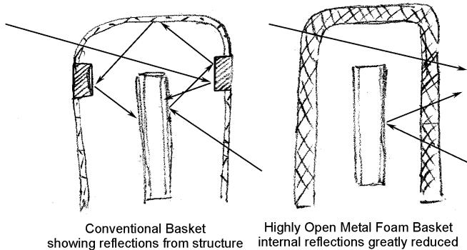
in the left picture. These reflections in turn introduce acoustic resonances in the microphone response which contribute to frequency response anomalies and
