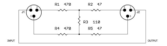
In either case, the performance of the microphone and that of the preamp are not compromised. The extra resistance in series with the signal does cause some extra noise, but at high signal levels this isn't typically a problem. High quality metal film resistors, preferably thin-film types, should be used to prevent any signal degradation.
